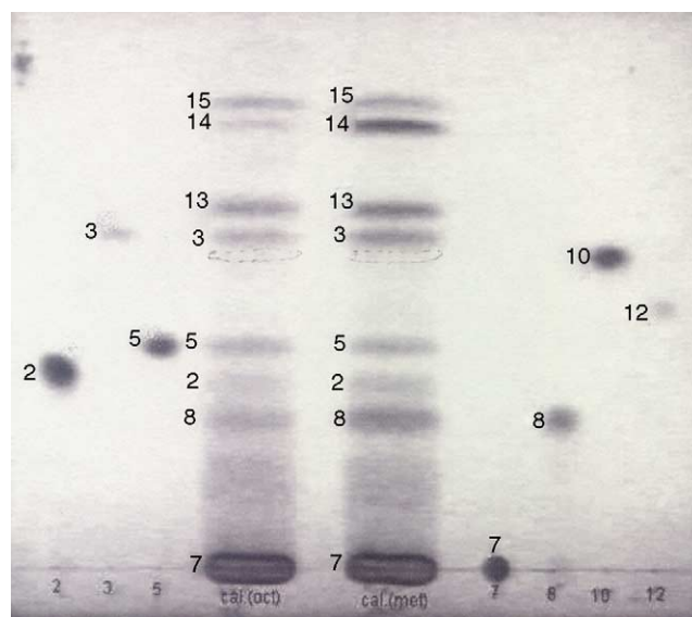
Fig. 5. Results from HPTLC of the ethyl acetate (cal.(oct)) and methanol (cal.(met)) extracts of C. officinalis flos —investigation of phenolic acids. Zone and standard no.: 2, protocatechuic acid; 3, vanillic acid; 5, syringic acid; 8, caffeic acid; 7, chlorogenic acid; 10, p -coumaric acid; 12, ferulic acid; 14, 15, not identified. Chromatographic system: Si60, mobile phase as in Table 1. Video documentation: ProViDoc-Desaga \lambda = 254 nm.
